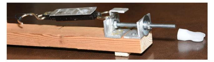
The picture above shows the system used to adjust the tension in the wire, a 100N spring balance indicating the tension.
