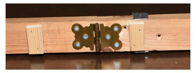
Since the hinge is on the underside of the body, four small pieces of wood were fixed to the body to act as feet and enable the body to sit flat on the table. Two of the feet are visible in the picture above, the other two are fitted at the ends.
