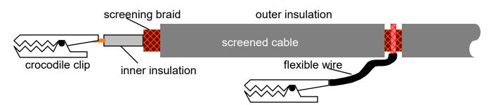
The screened cable extended the full length of the body and a crocodile clip attached to the inner conductor. The end of the screened cable is wrapped with 'gaffer' type tape to cover the screening braid and provide protection to the inner conductor. This crocodile clip was used to make a connection to the wire where it is secured to the body.
