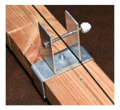
The moveable bridge was made from two bent pieces of aluminium, glued and bolted together.
