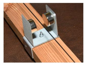
The magnet arrangement should be moveable so that it can be positioned near to the centre of the wire. This is where there will be the maximum movement of the wire and so the maximum voltage generated.
