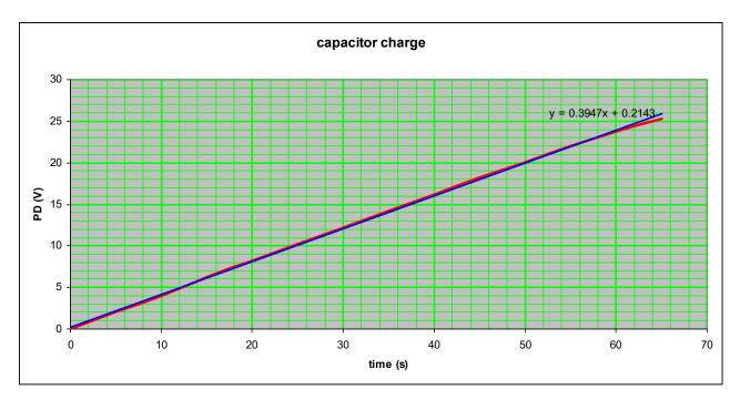
From the trend line, the gradient is  $0.395~Vs^{-1}$  => From eqn 1 C = I / gradient =  $0.36 \times 10^{-3} / 0.395 = 911 \mu F$  which is consistent with the measured value.
