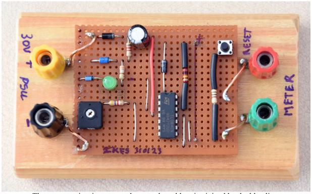
The test capacitor is connected across the solder pins joined by the blue line, with the positive side connected to the top (+) pin.
