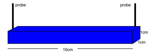
The probes from a digital voltmeter (DVM) were connected across the ends of the block. The meter displayed a '1' on all ranges!
