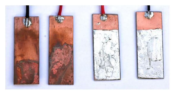
The electrical contacts for the Play-Doh were made from off cuts of printed circuit board. Lead free solder is mainly tin and so it is straightforward to melt lead free solder onto freshly cleaned copper on the circuit board to form tin plated contacts for the Play-Doh.
