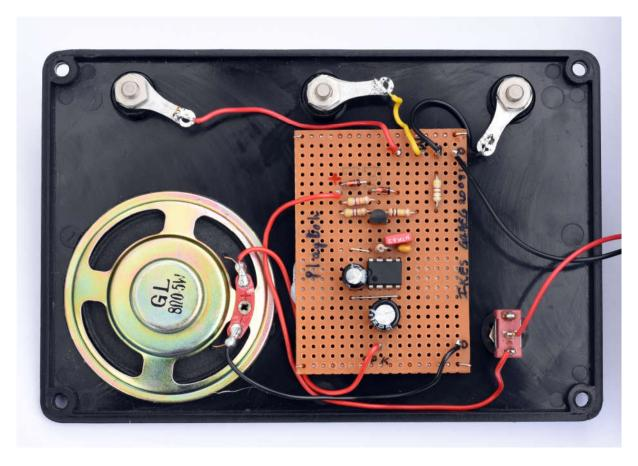
The red and black wires on the right hand side go to a PP3 battery. An On/Off switch is wired into the positive (red) lead from the battery. The connections to the Play-Doh are made via the 4mm connectors seen at the top of the picture, the middle one being the one for the probe.
