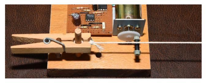
The photograph above shows how the string was attached to the motor vibrating board. A loop was tied into the end of the string and then passed over the wooden peg, secured in place by the clippeg. The position of the string should be so that the nylon bolt (just) hits the string when it is at the top of its rotation. The more the bolt touches the string, the larger the vibrations, but the more difficult the motor has turning slowly.
