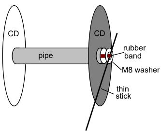
6). Wind up the rubber band in your roller using the thin stick. Place the roller on the table/floor and see if it moves. If it does not move, then wind it up more and try again.
