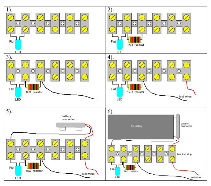
Connect the battery to the battery connector.
