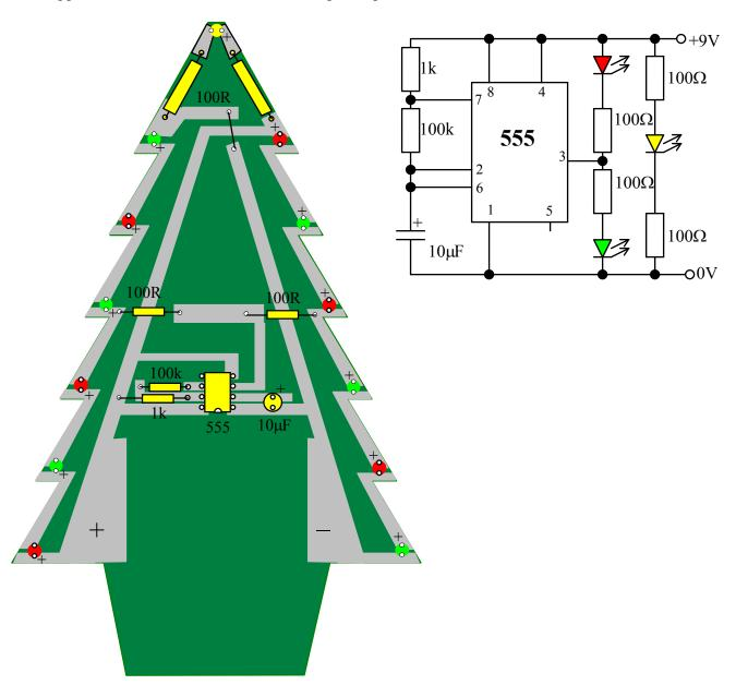
The pcb should be cut to the shape of the Christmas Tree prior to producing the copper tracks.
