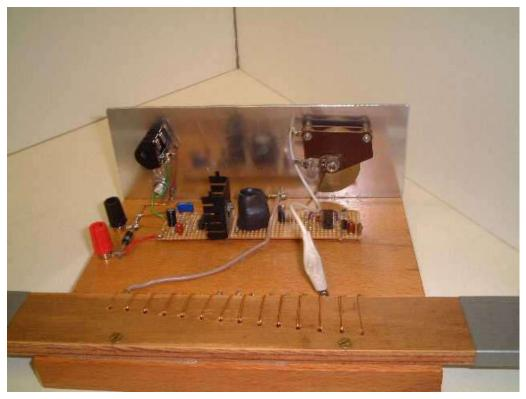
The Simple Loop Transmitter provides an easy way of generating an AM radio signal which can be used to demonstrate the principles of AM radio transmission and also provide a signal for a Simple Radio in the absence of a long wire aerial or nearby AM radio transmitter. The output power is
