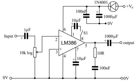
Switch S1 sets the gain:- open = 20 closed = 200. This is shown as a green solder blob below.
