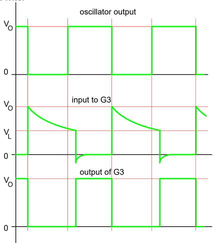
If R is the resistor at the input to G3, C is the capacitor from G2 to G3,  $V_0$  is the supply voltage,  $V_L$  is the lower switching voltage, then the time period of the unstable state is given by
