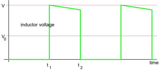
During this time, the battery and inductor must supply the energy to the load and also the energy to recharge the smoothing capacitor. Energy is also lost in the rectifier diode, which for a good Schottkey diode, can been ignored
