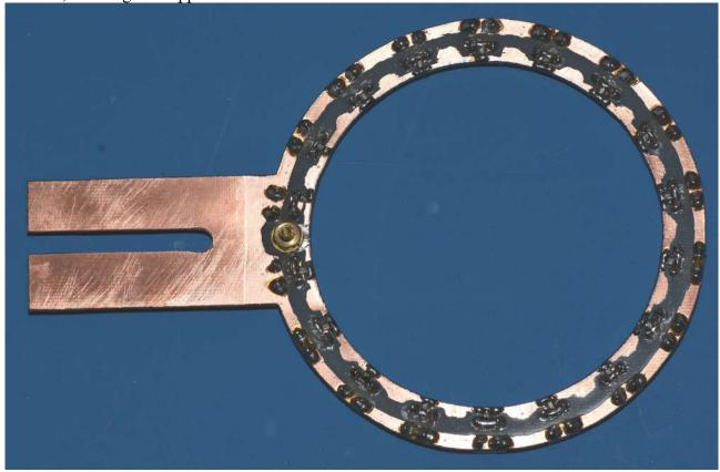
The ring lamp was cut from a  $100\text{mm} \times 160\text{mm}$  piece of fibre glass printed circuit board. It was helpful to draw concentric circles of the radius listed at the top of the diagram as a guide to marking out the copper track and position of the LEDs.
