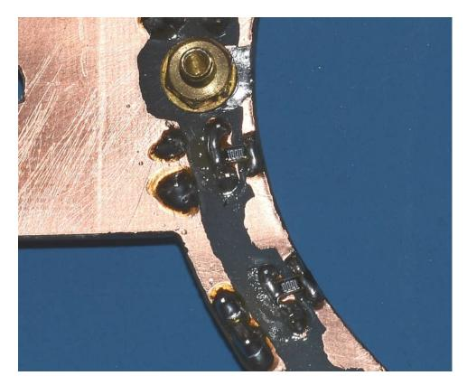
The LEDs are soldered in place, with the cathode (negative) to the outer ring. The  $100\Omega$  resistors are soldered between the anodes of the LEDs (positive) and the inner ring, as seen in the picture above. The connection to the inner ring was made from a brass 3.5mm (4BA) bolt, which was drilled in the centre to act as a socket for a 2mm plug. The copper board around the 3.5mm hole was coated in a thin layer of solder to ensure a good contact with the brass bolt.
