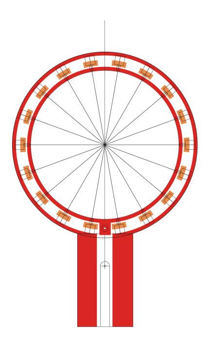
The inner and outer copper track width were 2mm and the sections of the middle track were 3mm wide.
