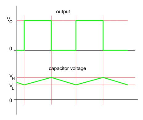
If R is the charge/discharge resistor, C is the capacitor,  $V_0$  is the supply voltage,  $V_H$  is the upper switching voltage,  $V_L$  is the lower switching voltage
