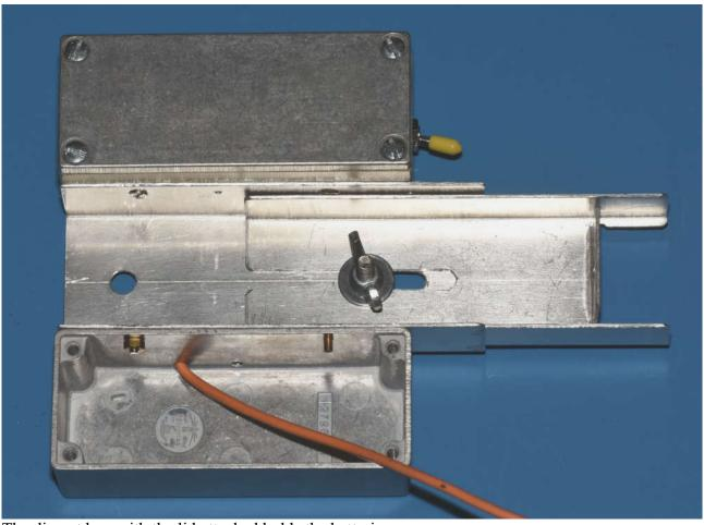
The diecast box with the lid attached holds the batteries.
