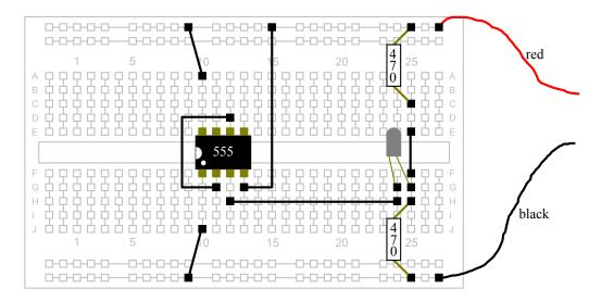
7). Connect a 47000 ohm  $(47k\Omega)$  resistor (Yellow, Violet, Orange, Gold) from pin 3 of the IC to column 5.
