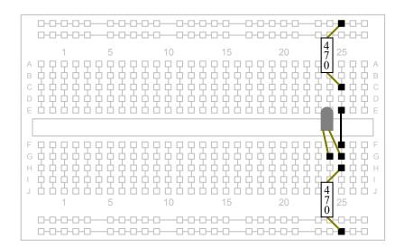
4). This section now needs to be tested. Connect the red lead of the battery connector to the top row and the black lead to the bottom row.
