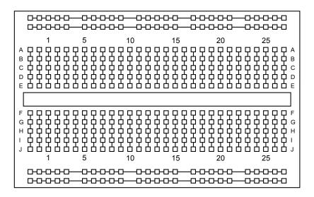
Note how each of the holes are connected.
