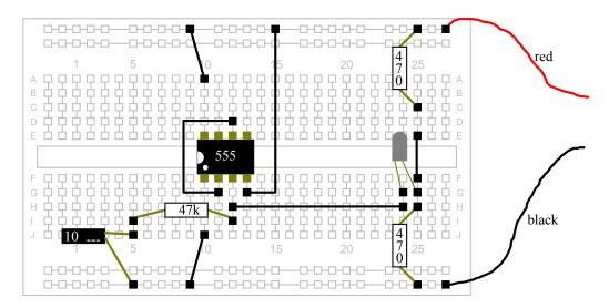
8). Connect a temporary wire from column 5 to pin 6 of the IC.
