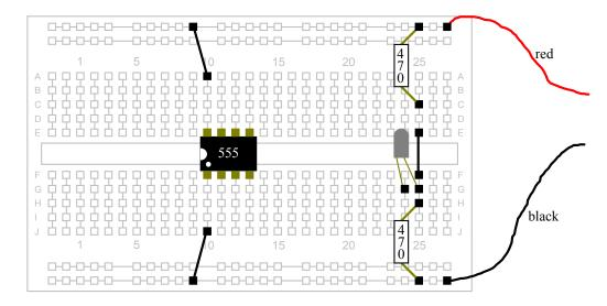
6). Connect a wire from pin 4 of the IC to the positive row. Connect a wire from pin 3 of the IC to the LED. Connect a wire from pin 2 of the IC to of the IC pin 6.
