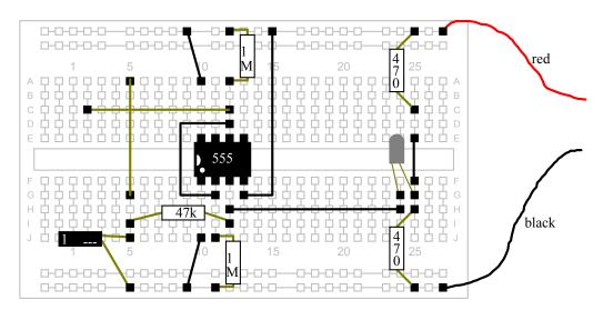
Reconnect the battery and the LED should glow either Red or Green. Push down where the bared wires cross and the LED should change colour.
