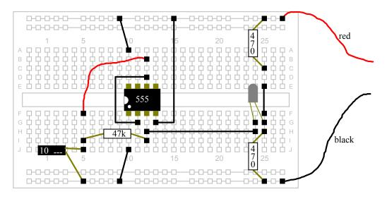
Connect the battery to the circuit.
