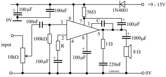
R sets the voltage gain (100 $\Omega$  ×50). C sets bandwidth (220pF 25 to 20kHz)
