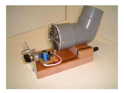
The speaker used was a 66mm device, mounted into a piece of drain pipe. This provides opportunities to demonstrate the effect of altering the loudspeaker enclosure.
