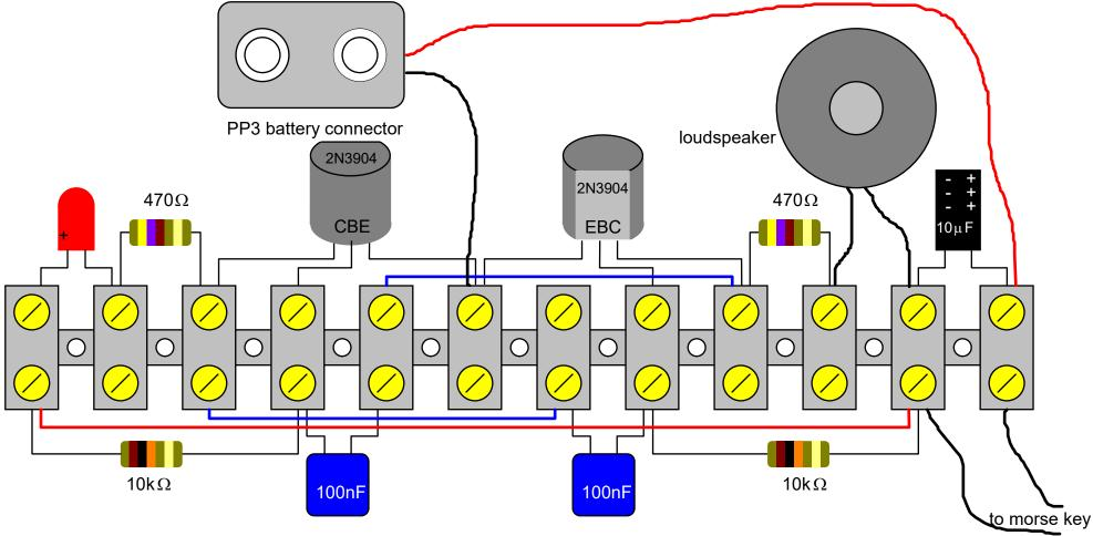
Connect the battery. If all is well, nothing will happen! Join the two wires together for the morse key and a tone should be heard from the loudspeaker and the LED should light. If it does not, then check your wiring for errors and also check that all of the wires are being held by the screws in the terminal strip.
