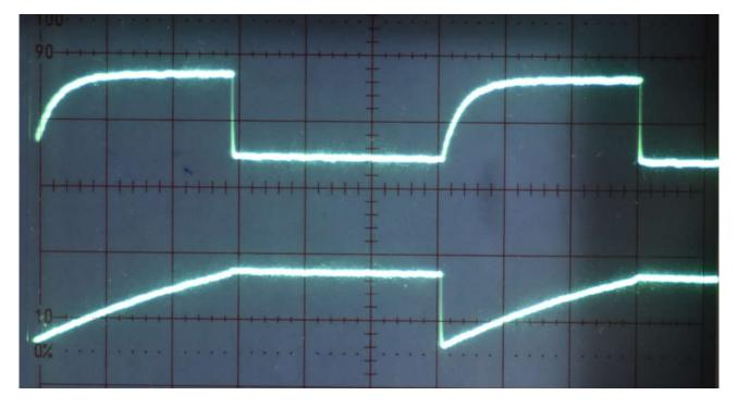
The picture above shows the collector voltage of TR1 (top) and the base voltage of TR1 (bottom). When TR1 is switched off (high voltage), the base voltage can be seen increasing slowly from a negative voltage to  $\approx 0.7$ V, at which time TR1 can be seen to quickly switch on (voltage goes low).
