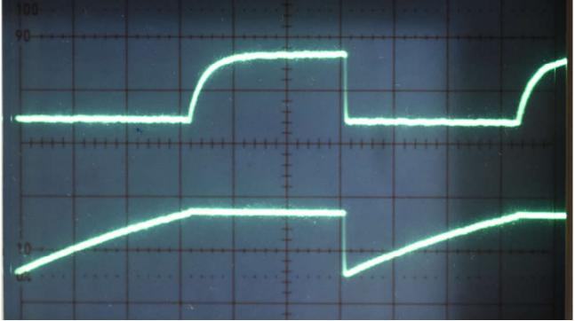
The picture above shows the collector voltage of TR1 (top) and the base voltage of TR2 (bottom). When TR1 is switched on (low voltage), the base voltage of TR2 can be seen to slowly increase from a negative value until it reaches  $\approx 0.7V$ , at which time TR1 starts to switch off and the voltage becomes high.
