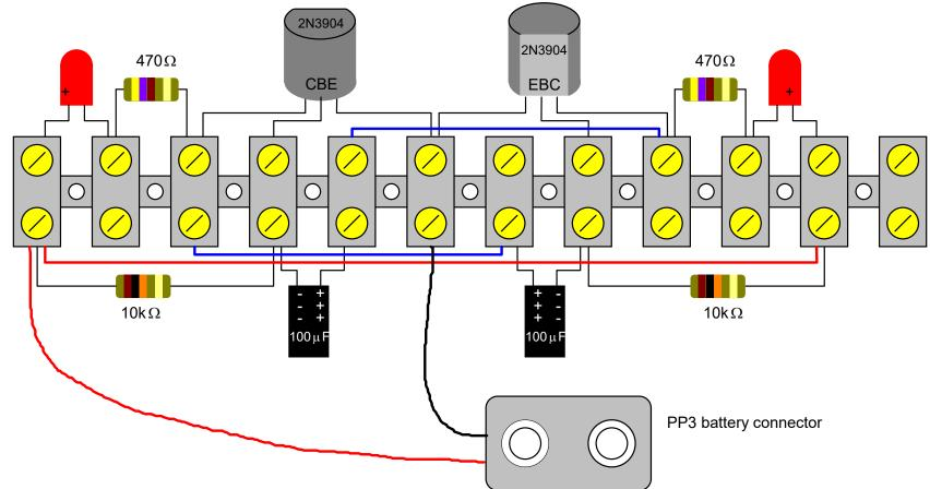
Connect the battery. If all is well, the LEDs will alternately light up. Secure your circuit and battery to the cardboard base with Sticky Tac to prevent it being damaged by being moved. If your circuit does not work, carefully check that there are no wiring errors and that all of the wires are secure in the terminal strip.
