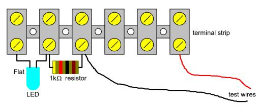
5). Take the battery connector and fit the black and red wires to the terminal strip as below. Carefully tighten the screws.
