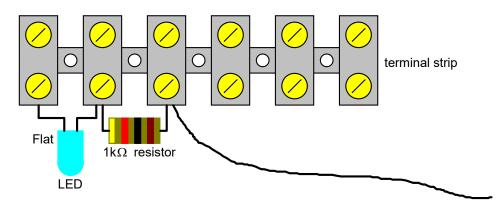
4). Take the red test wire and fit it to the terminal strip as below. Carefully tighten the screw.
