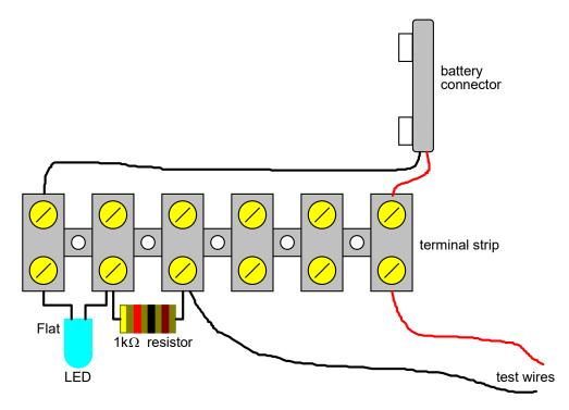
6). Connect the battery to the battery connector. Touch the test wires together.
