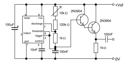
The frequency is tuned using the  $10k\Omega$  adjustable resistor. The frequency should be 116.5Hz.
