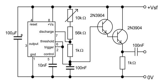
This is the same as the bass drone but with different timing resistors.
