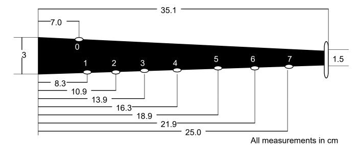
The diagram above show the measurements for a typical chanter. However, since the tuning is electronic, the actual sizes do not affect the pitch of the notes. The holes contained small tactile switches, wired through a hole running along the length of the chanter.
