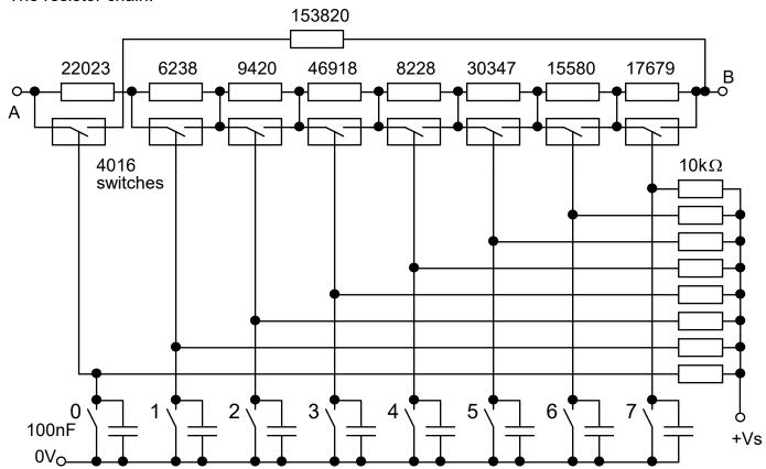
The switches on the chanter were small tactile (NO) switches. These were used to switch 4016 electronic switches and were debounced using the  $10k\Omega$  pull up resistors and the 100nF capacitors across each tactile switch.
