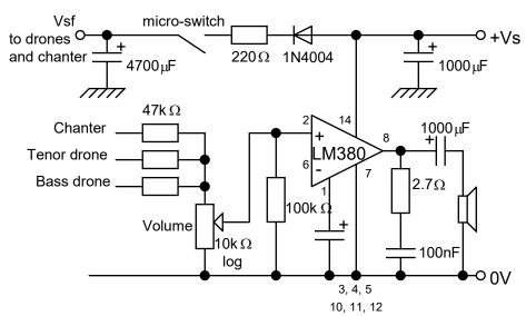
The output amplifier is a standard LM380 circuit which will deliver around 1W to an internal speaker.
