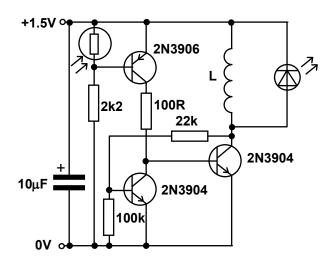
The LDR is an ORP12 type device and the 2k2 resistor can be adjusted to provide the required light level at which the LED will switch on.
