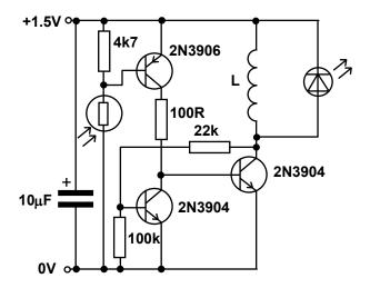
The LDR should be placed so that light from the LED can fall onto the LDR when it is lit. The LDR will need to be shielded from ambient light to ensure that it responds only to light from near the LED.
