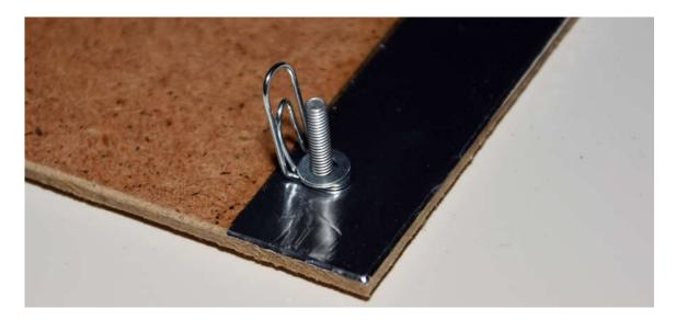
Carefully screw a nut onto the bolt. Hold the nut and paper clip with your finger and thumb of your left hand and **CAREFULLY** tighten the bolt with a screwdriver in your right hand.
