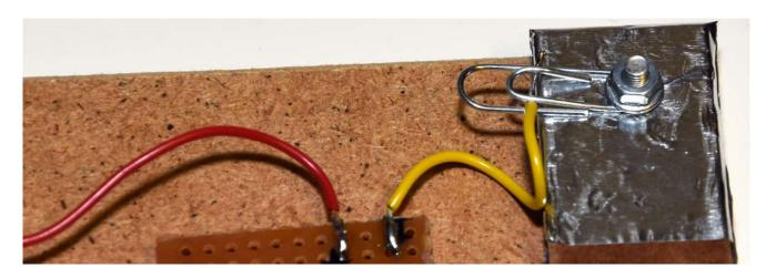
Put a small piece of Blu-tac under the oscillator to fix it to the baseboard. Put two small pieces of Blu-tac onto the baseboard where the AA cell fits. Put an AA cell in between the paper clips and push into the Blu-tac.
