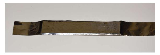
Turn the board over and put glue on each end of the board. Fold over the aluminium foil and stick on to the board. Ensure that the aluminium foil covers the hole in the board.
