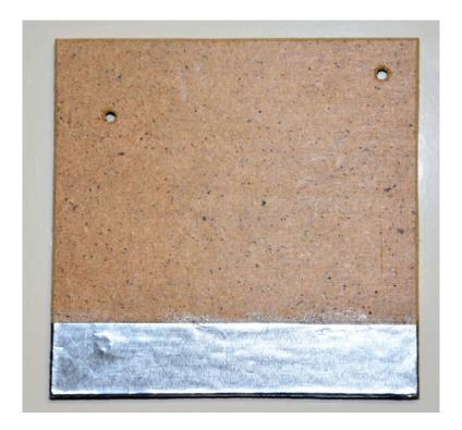
Carefully push the point of a pencil through the aluminium into the hole.
