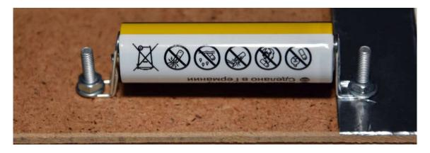
Put a bolt through the last hole in the base board and then fit the small, square piece of board onto the bolt.
