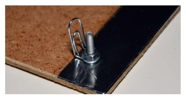
This makes the negative connection for the 'AA' cell.
