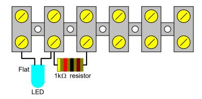
3). Take the black test wire and fit it to the terminal strip as below. Carefully tighten the third screw.
