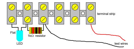
5). Take the battery connector and fit the black and red wires to the terminal strip as below.
