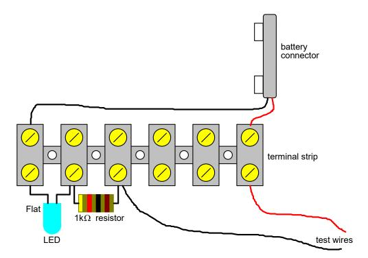
6). Connect the battery to the battery connector.
