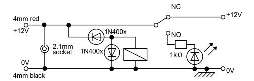
The relay has a 12V coil and 5A contacts. Under normal conditions, current flows through the normally closed (NC) relay contacts to the circuit.
