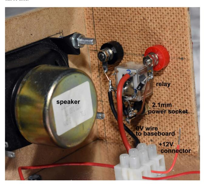
The 2.1mm power socket can just be seen in the picture above and is wired with the centre pin as positive, which is standard for many power-supplies.
