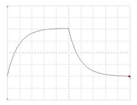
The charging section provides a suitable control voltage to operate the VCA, but the discharge section gives a click due to the very rapid initial discharge and so, in this form, is unsuitable. This charging/discharging waveform can be modified by using diodes and resistors to limit the maximum voltage. This is the same method that is used in many basic signal generators to produce a 'sine wave' output from a triangular waveform.
