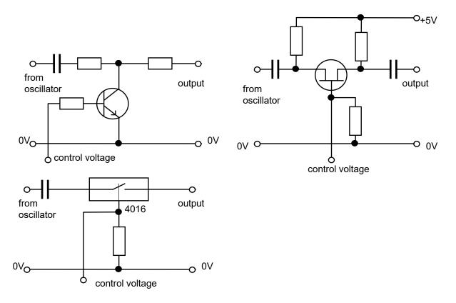
All of these circuits distorted the sine wave as the gain was reduced. Circuits requiring a negative power supply were rejected as were dedicated VCA ICs as these went against the principle of keeping the circuit simple.
