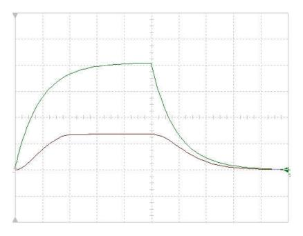
The capacitor charge/discharge is shown in green and the control voltage in brown.
