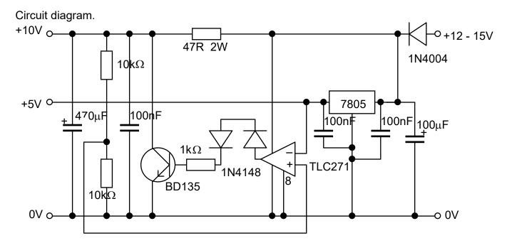
The BD135 and 7805 are both mounted on heatsinks.
