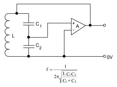
$C_1$  and  $C_2$  form a potential divider and it can be shown that for stable oscillation
