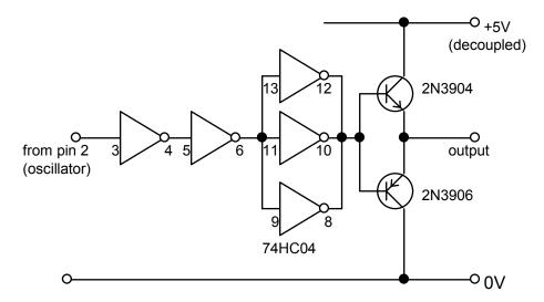
The +5V supply is decoupled with a 100nF ceramic capacitor and a  $10\mu$ F capacitor. This circuit has a frequency response beyond 20MHz (the limit of tests so far) and will supply an
