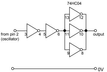
The NOT gates connected in parallel enable the buffer circuit to provide an output current of around 10mA. This can further be increased by adding a pnp and npn transistor pair as shown below.
