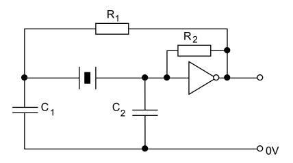
Crystals do not conduct, and so the NOT gate needs to be biased using a resistor,  $R_2$ . Many crystals will oscillate readily and so do not need a great deal of feedback to keep them in stable operation. A resistor,  $R_1$ , is therefore included in the feedback loop to the input of the crystal. The actual value of this resistor will need to be adjusted-on-test - the value chosen should be the largest value for which the crystal readily starts oscillating when power is applied.
