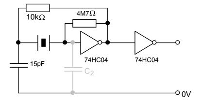
The capacitor  $C_2$  has been omitted, the input capacitance of the NOT gate providing sufficient capacitance for reliable oscillation.  $C_1$  can be a trimmer capacitor to allow the crystal frequency to be adjusted to a required value ( $\pm$  around 1kHz).
